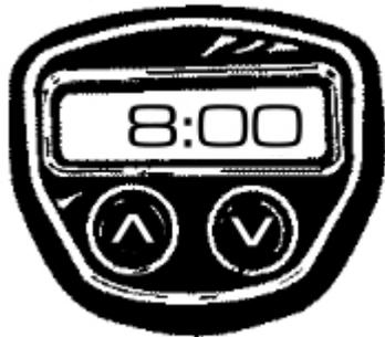
The screen will change and go back to this [ 3:00 ]. Pretty easy huh? The **Up-Arrow** increases the time, the **Down-Arrow** decreases the time. Press the **Up-Arrow** now, and hold it. The time should increase really fast. Keep holding it down until the display screen says [ 8:00 ]. If you go over, then use the **Down-Arrow** to adjust it.
